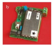
**Retransmission Module** (Iy) This 4-20 mA DC output board indicates valve position to the control
