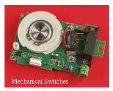
**Limit Switches** For cam activated indication of actuator travel limits, two output formats are offered: Mechanical Switches or intrinsically safe Inductive Proximity Switches (SIA) [not shown].
