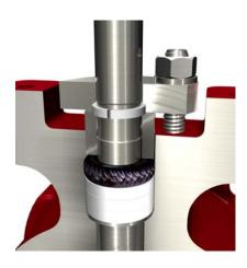
STEM SEAL: The stem seal system derived from the S40 provides a positive seal. PTFE packing seals the stem and a carbon fibre anti-extrusion ring contains the packing. Flexible graphite rings are available for high temperature applications. All Series 39 valves have one set of stem seal packing rings and a PTFE base cover gasket or O-ring seal in the body base.
