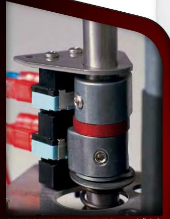
**CAMS/CAMS ADJUSTMENT** Cams are infinitely adjustable by the hex key with no special tools needed. Standard factory setting allows 90° reversible rotation between open and closed positions. Extended rotation such as 180°, 270° or beyond can be achieved simply by adjusting the cams.
