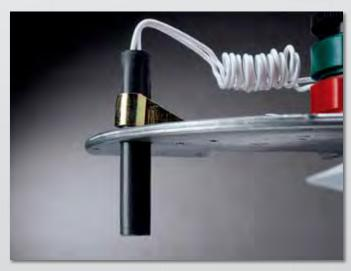
**HEATER:** A self regulating heater can be added to prevent possible damage to electrical components due to condensation build-up inside the actuator. Mounted in the actuator top plate for easy accessibility.
