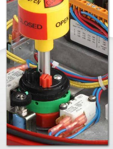
**AUXILIARY SWITCHES:** Independent dry-contact (voltage free) SPDT mechanical switches are available to indicate travel position to remote customer control systems.
